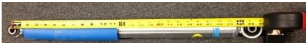
This shock has a length of approximately 25 inches. Measurement is taken from centre of eye to centre of eye.
