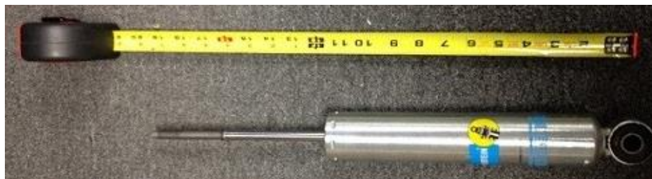
This shock has a length of approximately 16 inches because the measurement is taken to the base of the mount, where the threading starts
