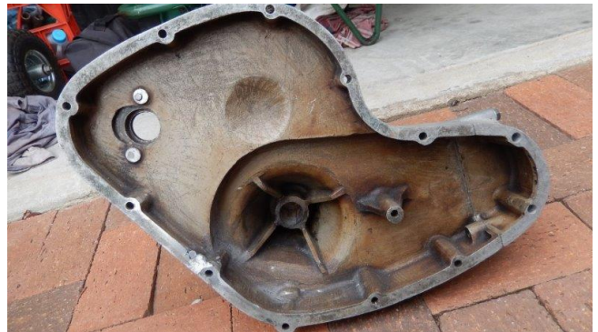
Above and below - the inside an outside of the front timing cover
